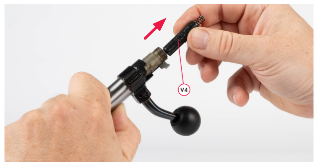
Fig. 16 Removing the rear spring support
