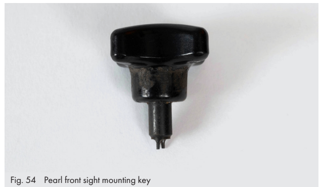
Fig. 54 Pearl front sight mounting key
