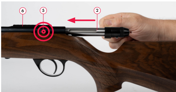
Fig. 7 Insert bolt[2] while pressing bolt catch [5]
