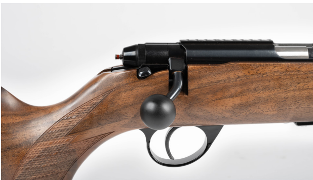
Fig. 28 The firearm is loaded, cocked, and the safety set
