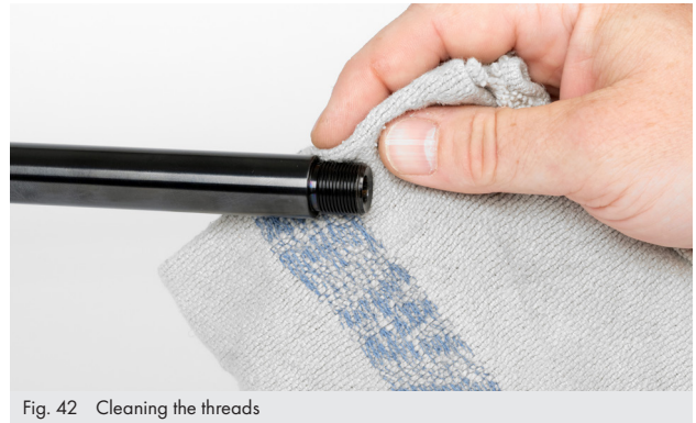
Fig. 42 Cleaning the threads
