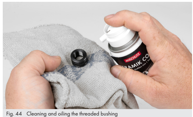
Fig. 44 Cleaning and oiling the threaded bushing
