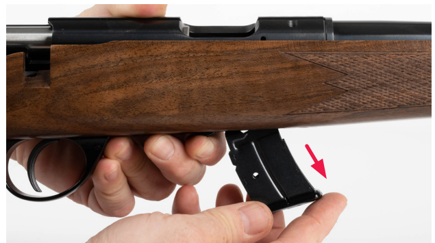
Fig. 22 Removing the magazine
