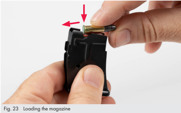
Fig. 23 Loading the magazine
