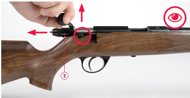
Fig. 29 Opening the bolt
