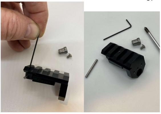
Place the scope mount where the Iron site was removed as shown.
