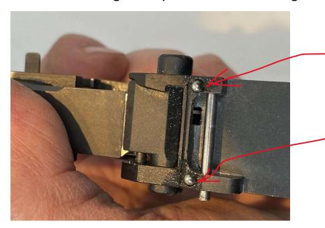
From the right side push the Iron sight retaining pivot pin by pushing it out with pin provided from the right to left.
