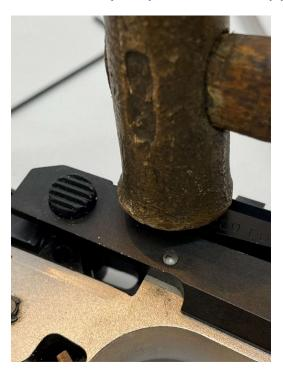
Push down the rear and install the large retaining pin. There should be a notch in the pin to indicate up or down. If the pin is hard in insert have the notch up. If it goes in real easy turn it and re-insert to get the snuggest fit.
