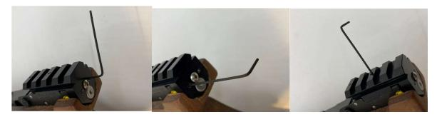
The mounting of the scope rail is complete.
