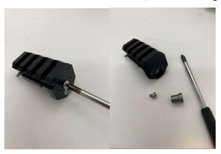
Loosen the front Allen screw that retains the front mounting pin.
