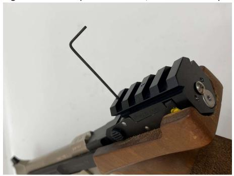
The following 3 Allen screws are just to remove any play and snug up the fit. These should tight but not be really tight.
