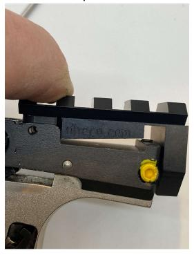
Install the front retaining pin provided. Center it in the frame.
