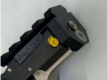
Note, the threaded hole in the rear of the large pin is to use when removing the mount, screw a 4-40 screw in and pull the screw to remove the pin.
