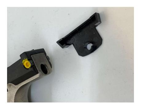
Step 3) Turn elevation screw clockwise to the stop (in the H direction) This relieves pressure on the springs under the sight.
