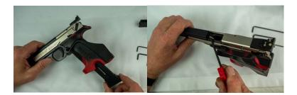
Step 2 – Remove dovetail cover by loosening the screw with 3mm allen wrench.
