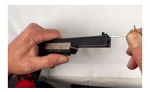
Step 4 – Install scope mount recoil lug into front sight post hole and tighten front sight retaining screw.
