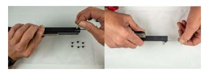
Step 5 – Slide scope mount dovetail adapter into dovetail on pistol.
